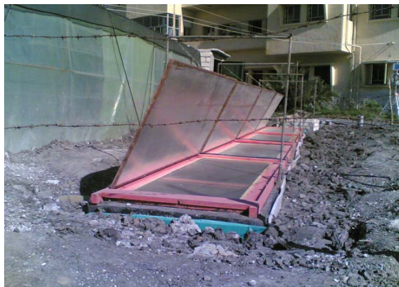
Fig. 2: The solar thermal system was opened from sunrise till sunset and the system covers were acted as solar reflectors during daytime and closed from sunset till the sunrise next day.
