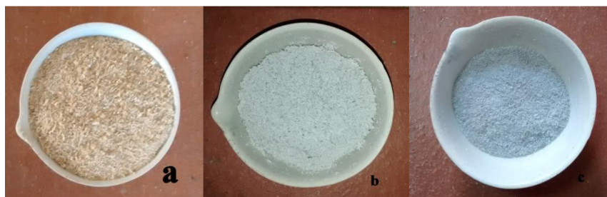
Fig. (1): Appearance of raw rice husk and extracted silica by different treatment schemes: a) raw rice husk, b) extracted silica by combustion of untreated rice husk at 600°C, and c) extracted silica from treated rice husk in H 2 SO 4 followed by combustion at 600°C
