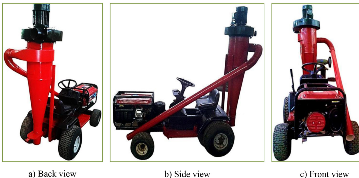
Fig. 2 The prototype view of jojoba seeds harvesting unit
